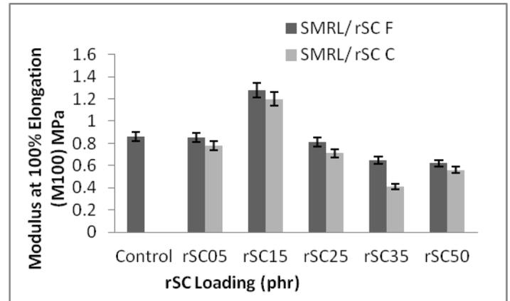
Fig. 2. Effect of rSC Loading on Modulus at 100% Elongation of SMR L/rSC Vulcanizates
