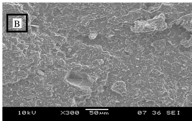
Fig. 4. SEM Micrographs of Tensile Fracture Surface of SMR L/rSC F (A) and SMR L/rSC C (B) Vulcanizate with 15phr of rSC Loading at 300X Magnification
