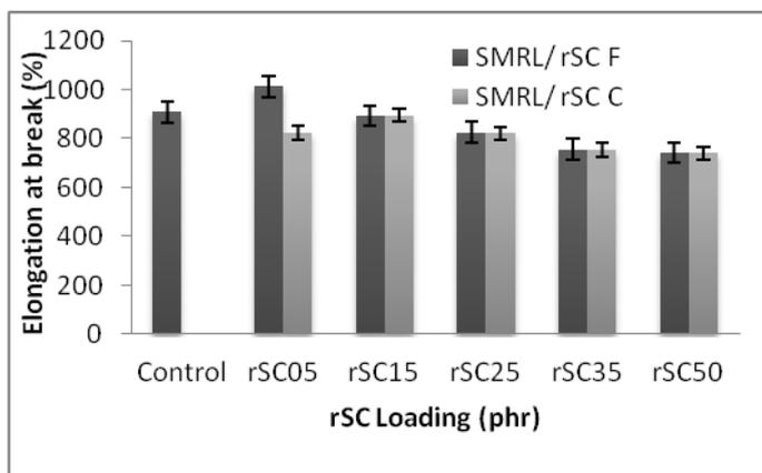
Fig. 3. Effect of rSC Loading on Elongation at Break of SMR L/rSC Vulcanizates
