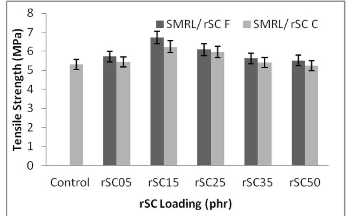
Fig. 1. Effect of rSC Loading on Tensile Strength of SMR L/rSC Vulcanizates
