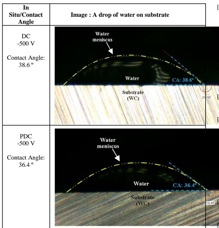
Fig. 3: Water drop wetting ability of WC substrate at DC -500 V and PDC -500 V
