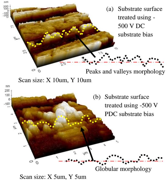
Fig.2: AFM three-dimensional images of WC substrate surface inspected area formerly treated by (a) DC and (b) PDC substrate biases
