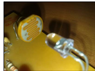
Figure 6. The LDR and LED work together
