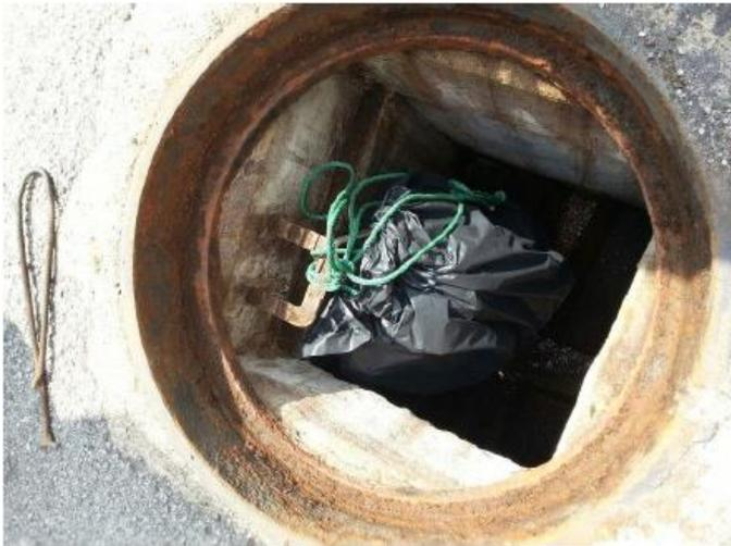
Fig. 2. Main flowmeter unit attached to handhold in manhole
