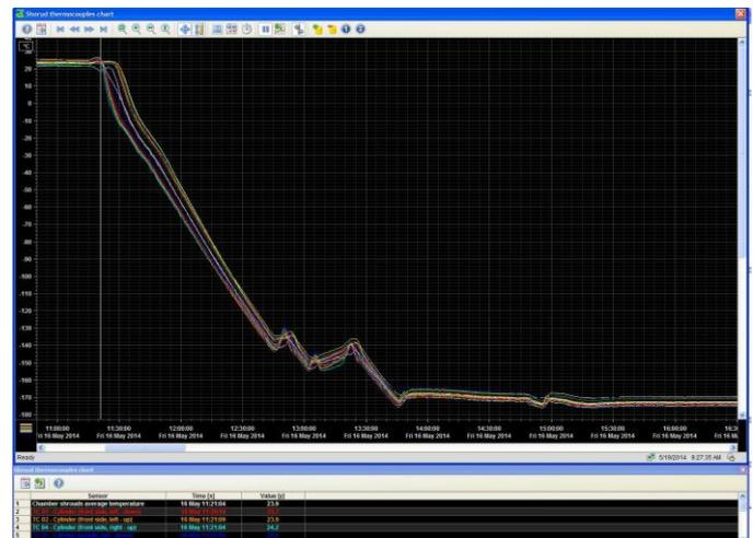
Fig. 5. Test Temp. Range GN2 for -173°C to 150 °C
