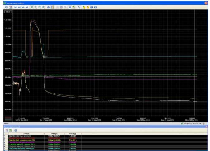
Fig. 3. Ultimate Vacuum Test 10<sup>-7</sup>mbar
