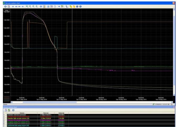
Fig. 4. Ultimate Vacuum Test 10<sup>-6</sup>mbar within 5 hours.
