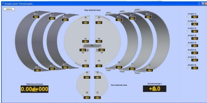
Fig. 2. Location of 20Nr. Thermocouple at the shroud inside the Chamber
