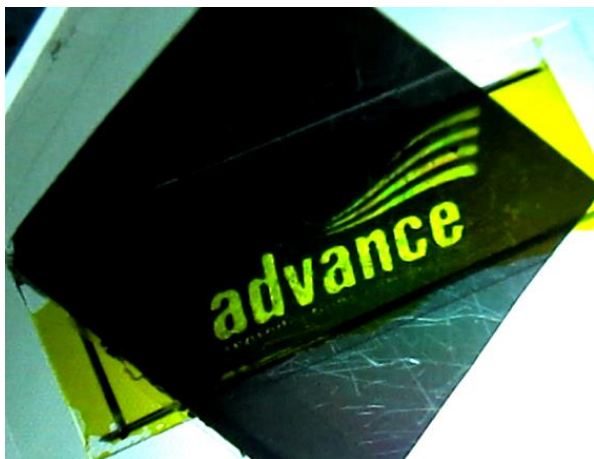
Fig.7: Demonstration of the permanent optical storage device made up of kojic acid based azobenzene moiety exhibiting photocrosslinking effect. Bright regions were masked and dark regions were illuminated. System changes from order to disorder transition.
